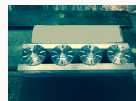
Slotting in mill, 4 pieces at a time saves time & cost
