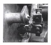
The yellow wire on the left side runs to your points and should connect there with the condenser as shown in picture #2. Using a new condenser not only simplifies installation it's also required for warranty.
